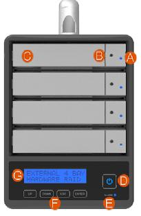
A. HDD Status Indicator LED E. Alarm indicator
